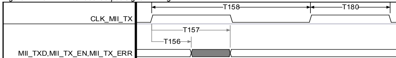
Figure 14-15. MII Interface Output Signal Timing
